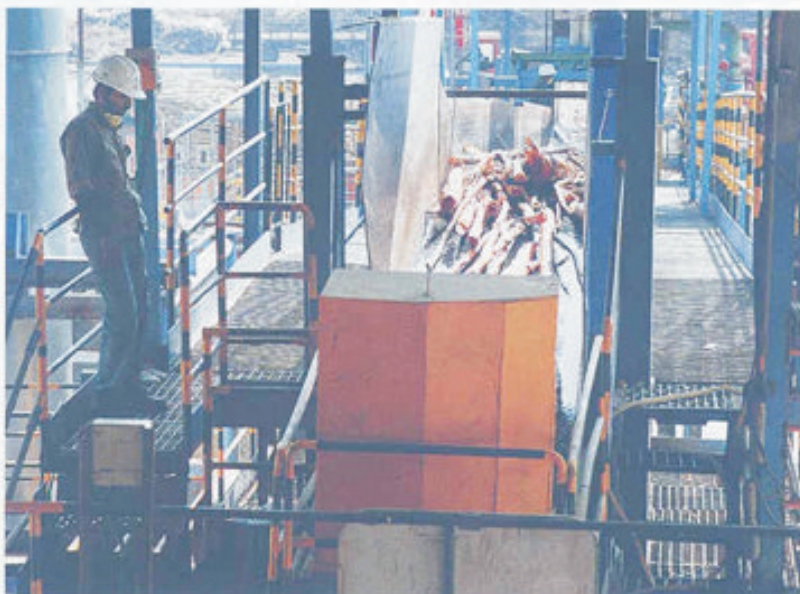
Wood being fed into a disc chipper, which cuts it to chips measuring 20 mm in size before being fed into the chip digester
